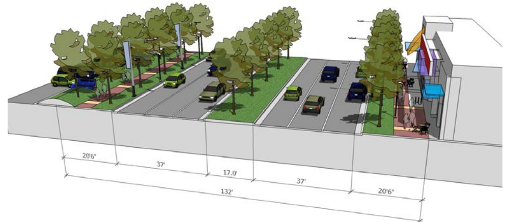
Figure 2.4 (2). Typical Cross Section Boulevard (State Street)
