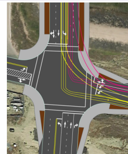
OSOW Accommodations at Signalized Gowen Road/Orchard Street
